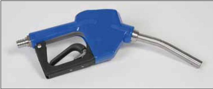
Mod. 729/AdBlue Automatic UREA-AdBlue nozzle • with swivel connector • INOX hose connector ext.diam.20mm Max flow rate: 40L/Min. (do not use for gravity)
