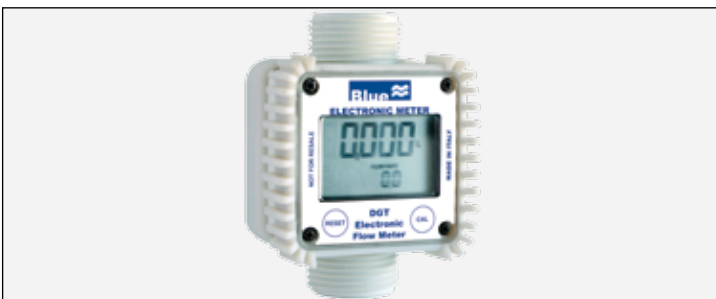
Mod. DGT3000 UREA-AdBlue Electronic flow meter Inlet/Outlet: 1" M + INOX Female connection 1" Flow rate: Min.6L/Min. - Max.100L/Min. Max pressure: 10bar Display: partial 5 digits - total 6 digits Frontal display can be differently positioned
