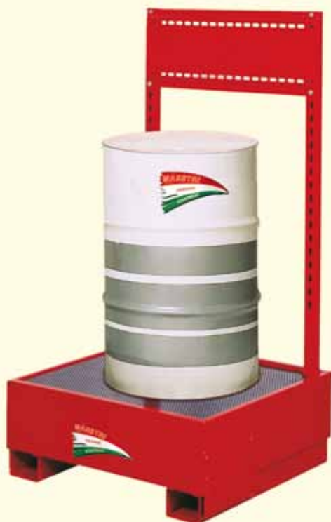
Mod. BASE 1 COMP Tank base for one 200kg drum with drilled steel plate and posts Capacity: 208L - Measure: 92x83x230cm Weight: 80Kg
